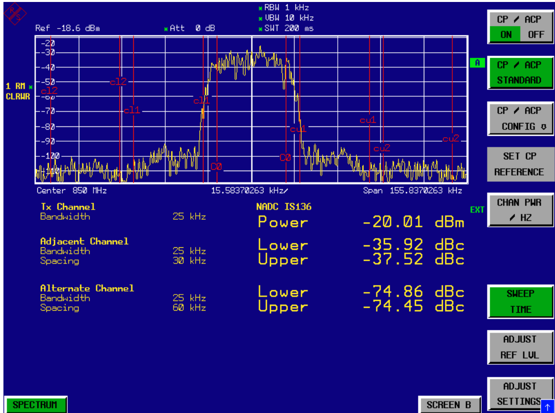
Fig. 2.35 Measuring the relative adjacent channel power of an NADC signal in each of the two adjacent channels below and above the transmit channel.
